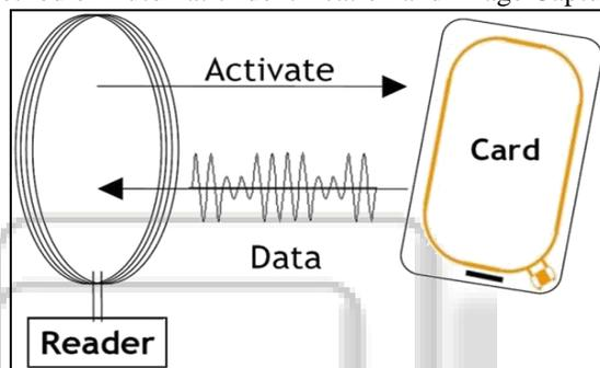
Fig 3.5. Working Process of RFID Cards
