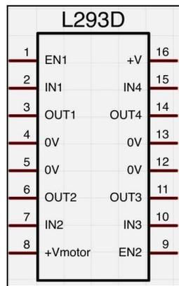
Fig. 3.4: Pin diagram of L293D
