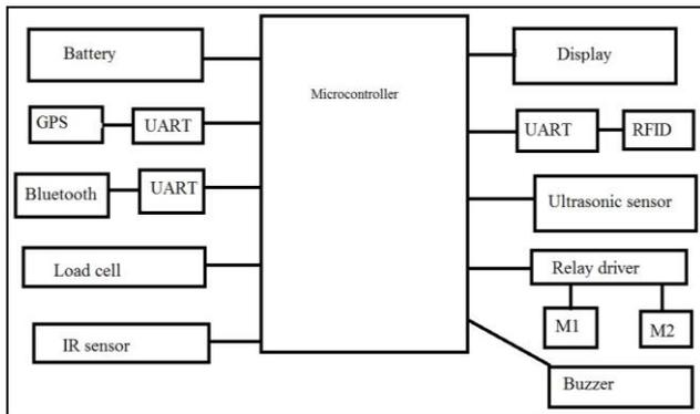
Fig. 2.1: Block Diagram of Intelligent Suitcase
