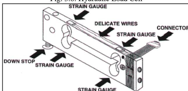
Fig. 3.7: Strain Guage Load Cell
