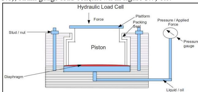
Fig. 3.6: Hydraulic Load Cell
