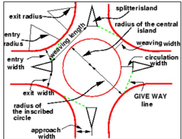
Fig. 1: Layout of General Rotary Intersection
