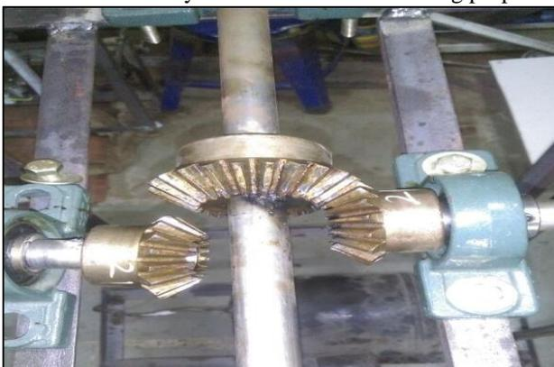
Fig. 4: Bevel Gear Arrangement
