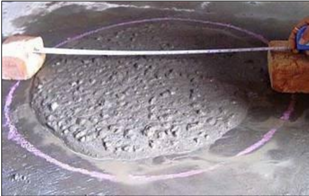
Fig. 2: Slump flow test and T 50 cm test
