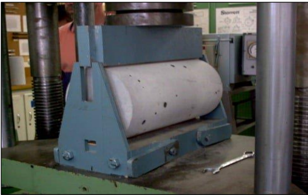
Fig. 4: Indirect Tensile Test
