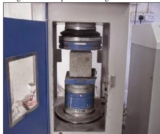
Fig. 3: compressive strength test
