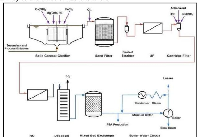
Fig. 3: PRE-WRP Process Flow Diagram
