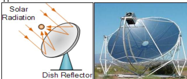
Fig. 5: Parabolic Dish Collector
