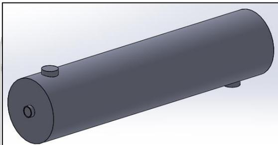
Fig. 1.3: Shell & Tube Heat Exchanger in Solid Model
