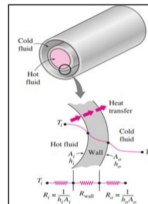
Fig. 1.2: Thermal Resistance Network Associated with Heat Transfer in a Double-Pipe Heat Exchanger
