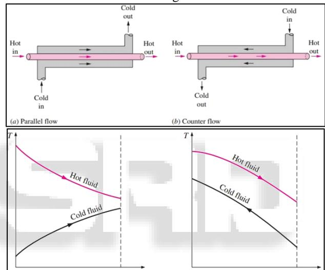
Fig. 1.1: Hot and Cold Fluid, Graphical Representations
