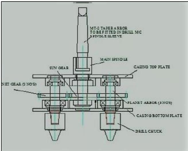
Fig. 1: Principle of twin spindle drilling
