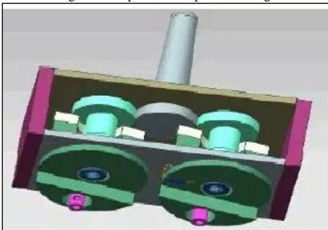
Fig. 2: Principle of twin spindle drilling in 2D
