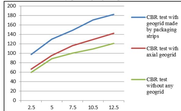
Fig. 4.1: Graph showing Load on Proving Ring vs Penetration on Plunger
