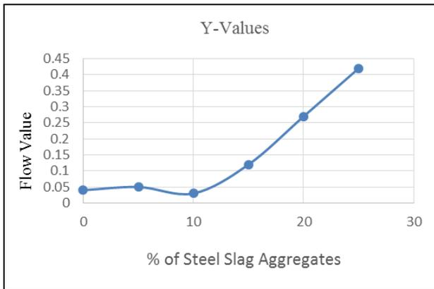
From this graph it is analyzed that the optimum percentage of replacement of conventional aggregate by steel slag aggregate is found to be 10%. This ratio of mix proves to be durable and cost effective.
