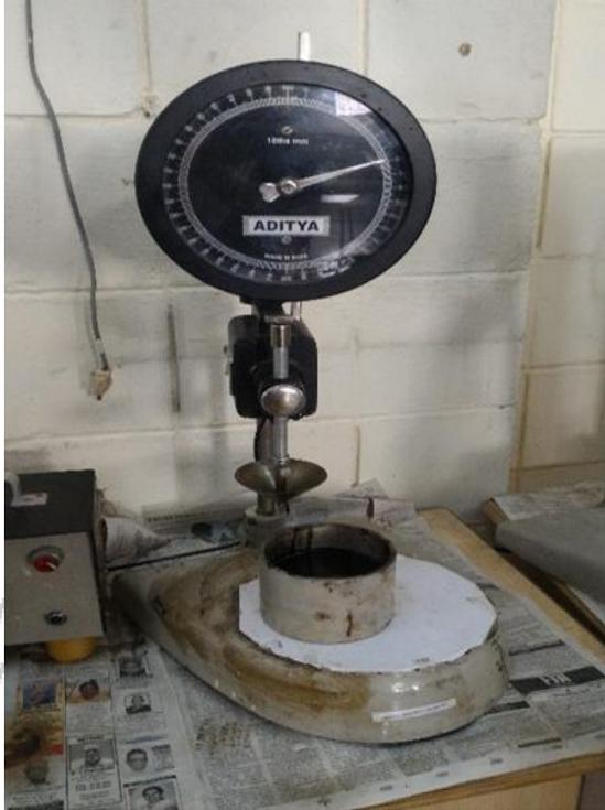
The average penetration value of a given bitumen sample is 58 and therefore the grade of bitumen is 60/70.
