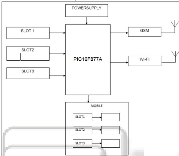
Fig. 1: Block diagram of smart parking system
