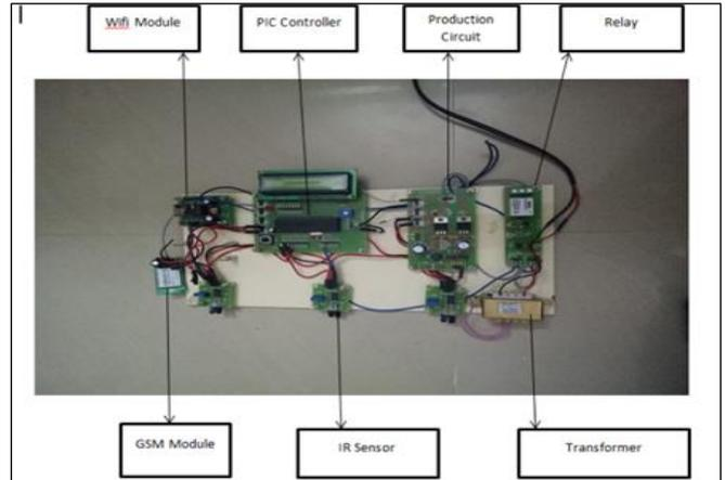
Fig. 6: Hardware setup in parking system
