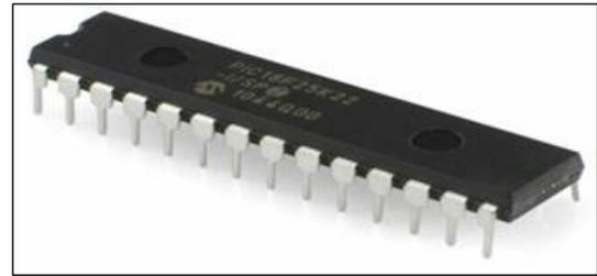
Fig. 2: PIC Microcontroller
