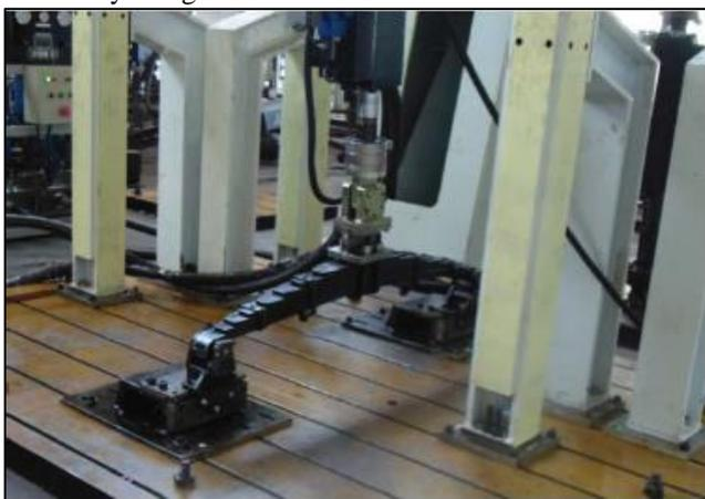
From this literature we studied the boundary conditions for testing machine are In rig test, Leaf spring suspension bracket were considered rigidly connected to the test bed with rotational bushes at leaf end & shackle. Therefore in simulation, the ends are fixed in all degrees of freedom except rotation about X-Axis. After the bolt
