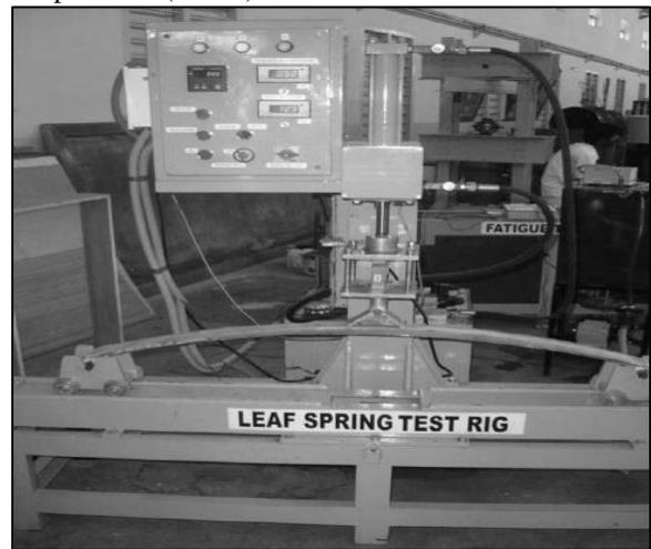
Important observation is, It includes static test, fatigue test, macroscopic inspection and metallographic analysis of leaf spring. For the static test, specimens are tested on Universal testing machine (UTM) and numerical analysis is done via (FEA) using ANSYS software.
