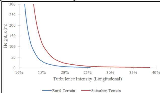
Fig. 5: Longitudinal Turbulence Intensity for Rural Terrain ( $z_0=0.04$  m) and Suburban Terrain ( $z_0=0.15$  m)
