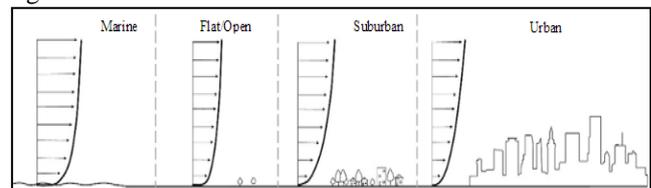
Fig. 2: Wind Profile in Different Boundary Layers
