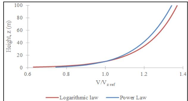
Fig. 3: Comparison of the Logarithmic and Power Law for mean Velocity Profile for  $z_0 = 0.02$  m and  $\alpha = 0.128$
