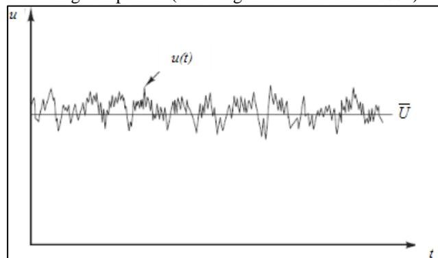
Fig. 4: Typical Point Velocity Measurements in Turbulent Flow
