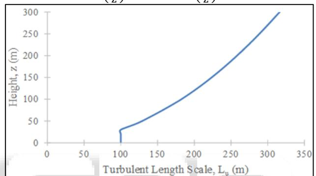
Fig. 6: Variation of turbulent length scale as height increases
