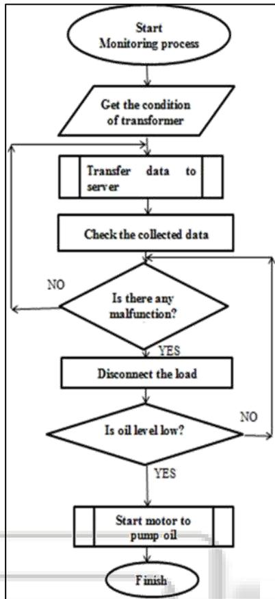
Fig. 1: Flow Chart of Monitoring System
