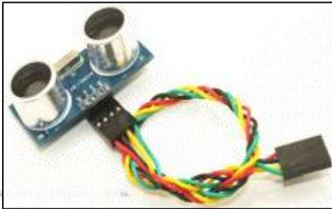
Fig. 6: Ultrasonic Sensor
