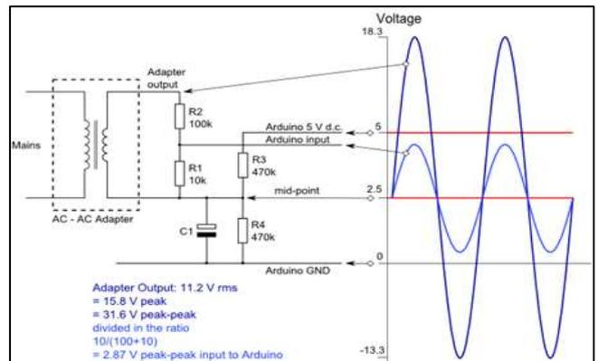
Fig. 4: Voltage Divider Circuit
