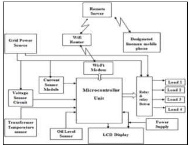
Fig. 2: Block Diagram of IoT based Transformer Condition Monitoring System
