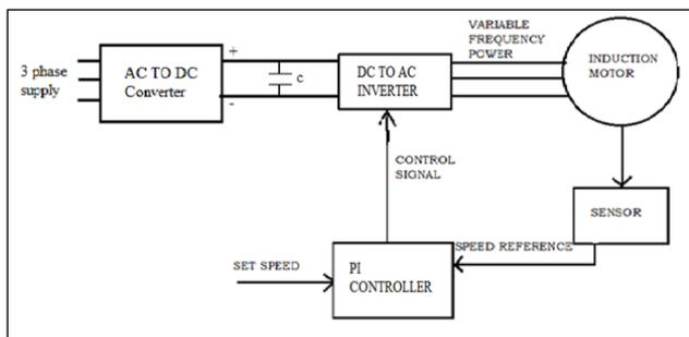
Fig. 1: Speed control of IM using PI Controller
