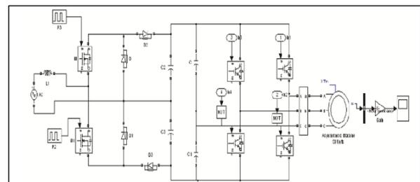
Fig. 3: Four Switch Three Phase Inverter Fed Induction Motor System with Half Bridge Doubler Boost Converter
