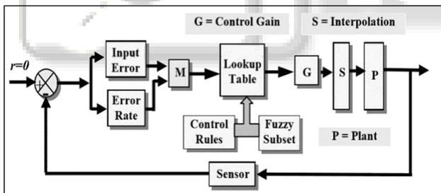
Fig. 4: Block diagram of Fuzzy logic controller
