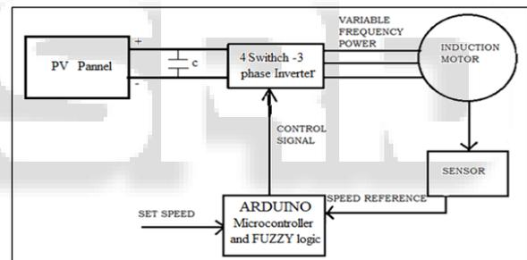
Fig. 2: speed control of IM using Arduino Micro controller and FUZZY logic
