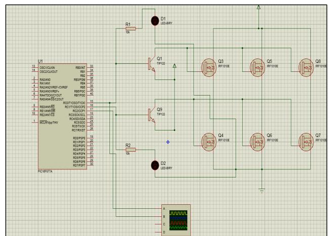
Fig. 6: Simulation of the Speed control of 4 Switch 3phase Inverter connected IM using Arduino Microcontroller and Fuzzy logic
