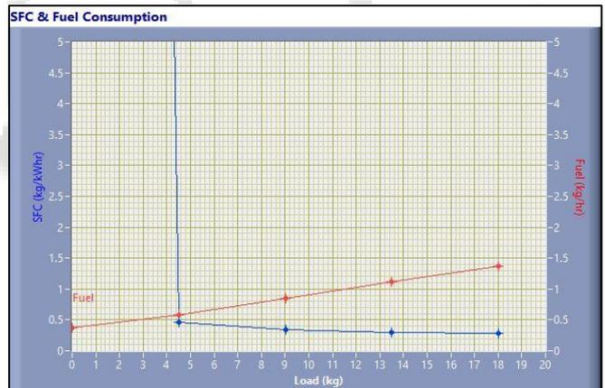
In the graph the results about the specific fuel consumption and fuel consumption. Load Vs specific fuel consumption and fuel consumption. Here load increased as well as fuel consumption also increased.
