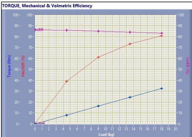
In this graph shown about the graph of torque, mechanical and volumetric efficiency. Specimen 1 and specimen 2 are shown the similar graph, so we take the result from that,
