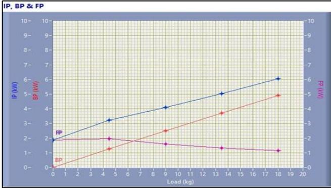
Three different B40 specimen has taken and conducted compression test for to identify the compression strength in the specimen. The graph shown, Load Vs Brake power, the load increased proportionally break power will increased and vice vesa. Similarly, load Vs indicated power and load Vs Feed power are also shown in the graph. It's also load increased gradually indicated power also increased and feed power.
