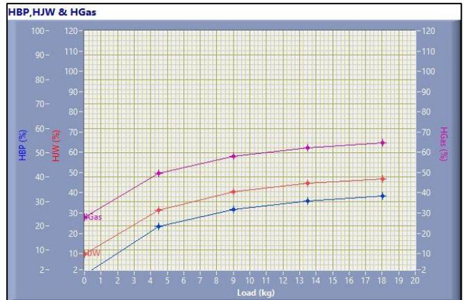
In this graph shown, load Vs heat brake power, heat water jacket and heat exhaust gas. First specimen shown load gradually increased at the time heat brake power and heat water jacket increased. Second specimen shown load increased from initially, heat brake power and heat water jacket start from near 10 Kw.
