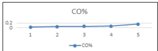
CO emissions at different idling conditions for diesel and biodiesel blend. The lowest CO emission is achieved for B40 at all the operating conditions. Also, in every condition diesel fuel produced maximum emission. As blend percentage of biodiesel in diesel increased emission decreased, this may be due to the higher concentration of O<sub>2</sub> in the air-fuel mixture which ensured improved combustion
