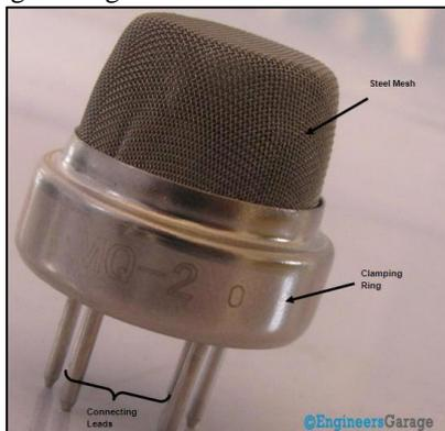
Fig. 4: MQ 6 Gas Sensor
