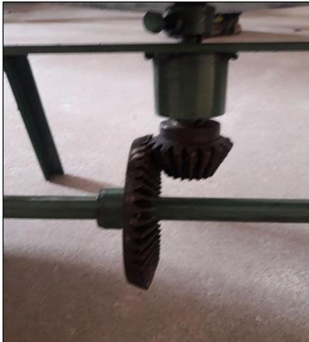
Fig. 2: Bevel Gear
