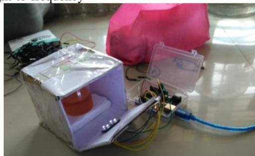
Fig. 7: TCS3200 Sensing A Colour For Soil Nutrition.
