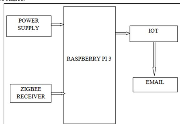
Fig. 1.2: Block diagram of receiving section
