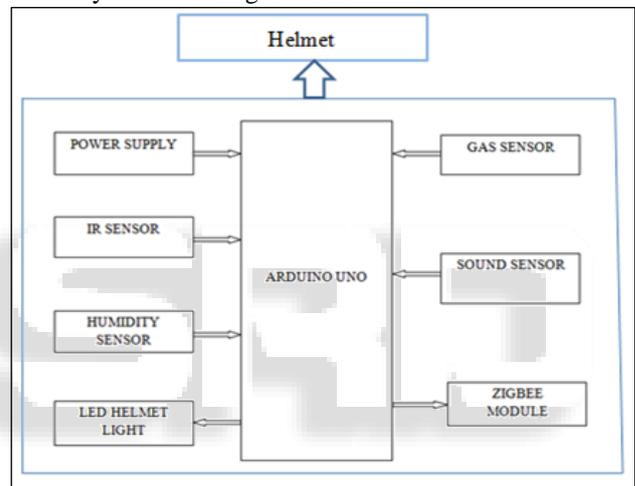
Fig. 1.1: Block Diagram of Transmitter section
