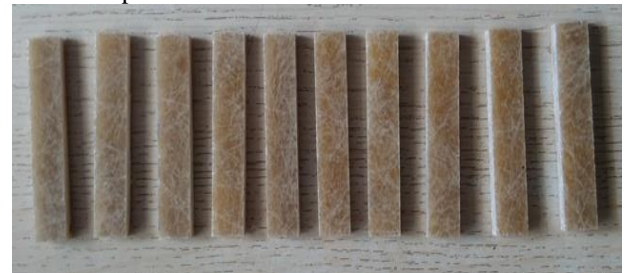
Fig. 7: Impact Strength Test Samples
