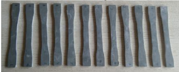
Fig. 5: Tensile strength test samples
