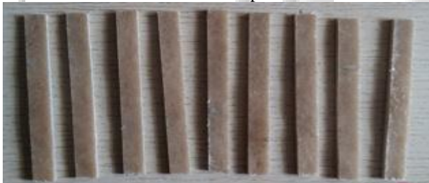
Fig. 6: Flexural Strength Test Samples
