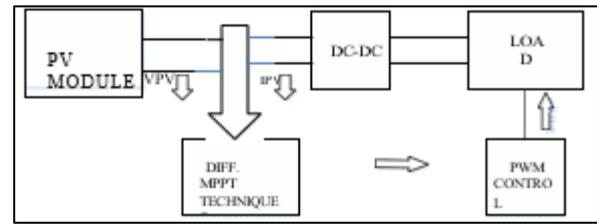
Fig. 3: Block diagram of the DC-DC converter for MPP operation
