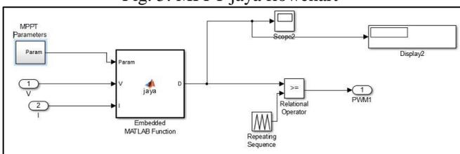
Fig. 6: Simulink model of Jaya algorithm
