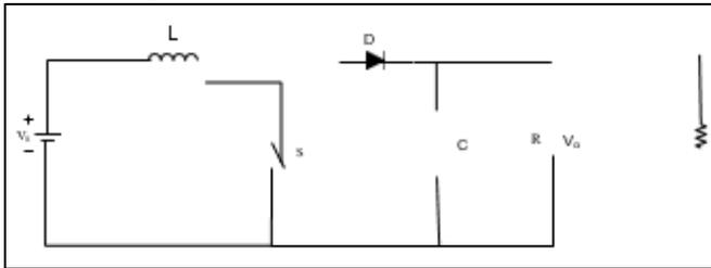
Fig. 4: DC to DC boost converter configuration
