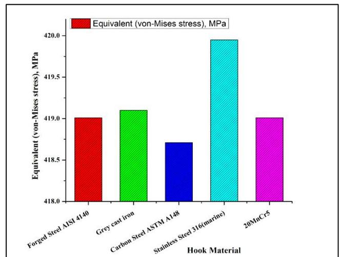
Fig. 5: Effect of Hook material on Equivalent (von-Mises Stress)
