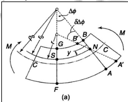
Fig. 2: Geometry of Bending of Curved Beam
