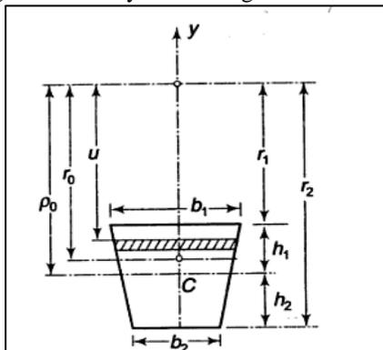
Fig. 3: Parameters for a hook Section
