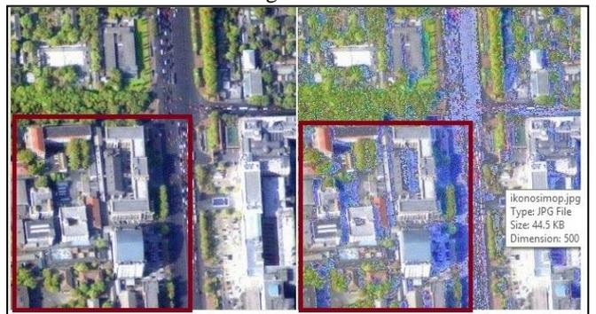
Fig. 6.12 (a): Original Image by IKONOS image with Shadow, (b) Recovered Image with Non Shadow
