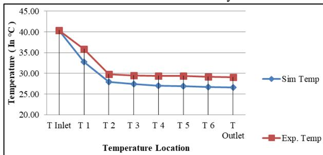
Fig. 7: Comparison of Simulated Temperature & Experimental Temperature at 5m/s Air Flow Velocity
