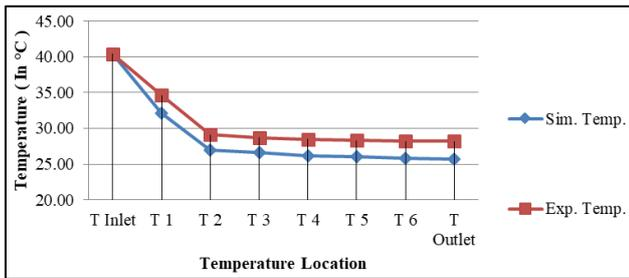
Fig. 6: Comparison between Sim. Temp. and Exp. Temp. at 3.5m/s Air Flow velocity
