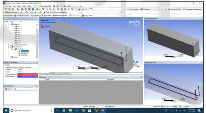
Fig. 2: Contact Surface between Soil & Pipe
