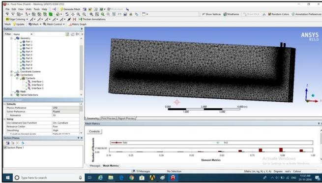
Fig. 3: Meshing of the GATHE at Pipe Section
