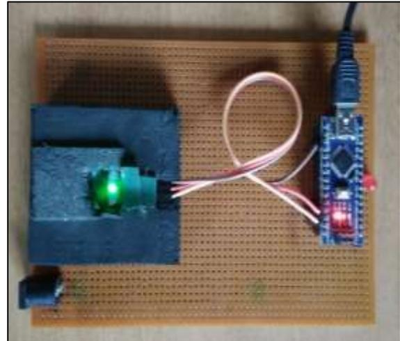
Fig. 2: Configuration of pulse rate sensor with Arduino
