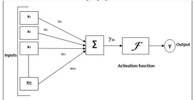
Fig. 4: Basic Model of Neuron Using Back Propagation
