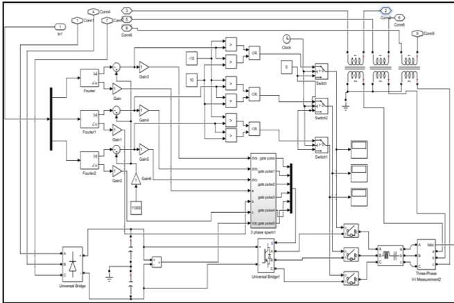
Fig. 7: Control Logic Implementation of DVR
