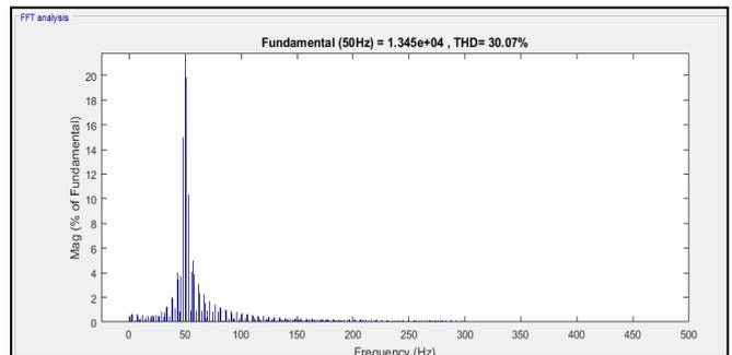
Fig. 5: FFT Analysis of Voltage without DVR
