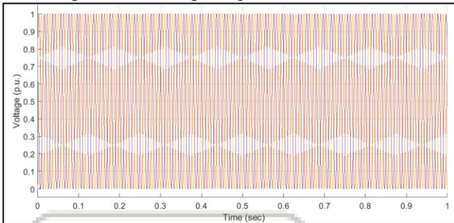
Fig. 8: Voltage Profile with DVR
