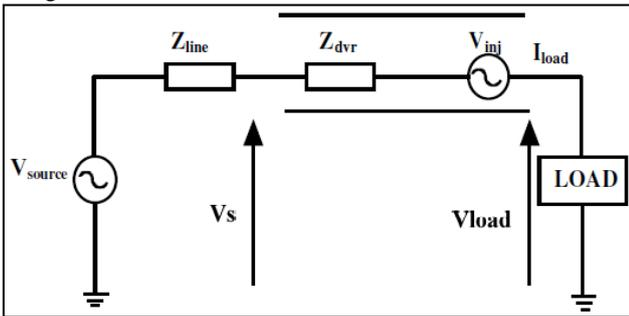
Fig. 2: Equivalent Circuit of DVR
