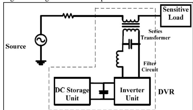
Fig. 1: Basic Structure of DVR
