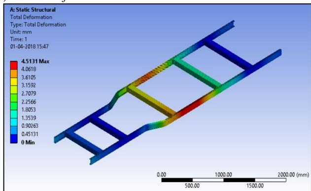
Fig. 10: Total Deformation
