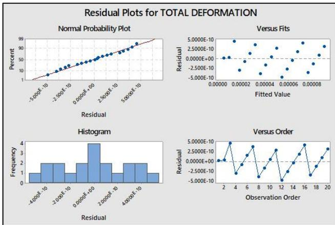
Fig. 7: Residual Plot for Maximum Total Deformation for Suspension Clamp
