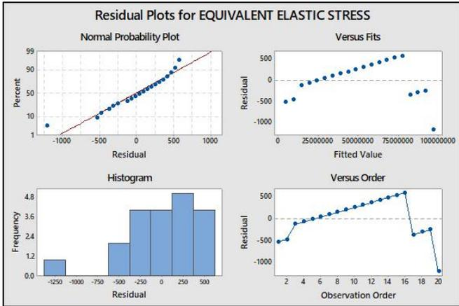
Fig. 1: Residual Plot for Equivalent Maximum Stress for Suspension Spring
