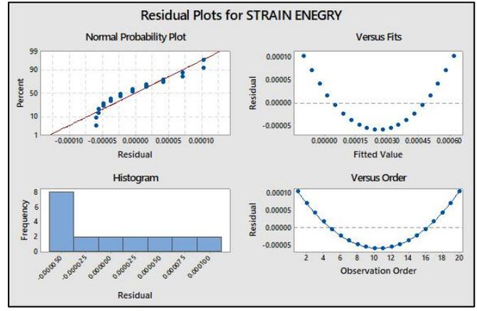
Fig. 4: Residual Plot for Strain Energy for Suspension Spring
