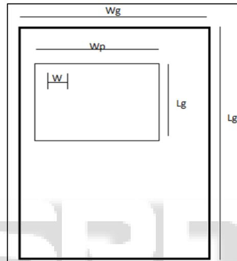
Fig. 5.1: Proposed Model of 2.4GHz Single Band Antenna
