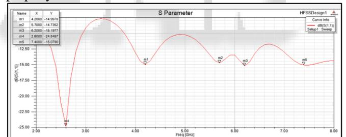
Fig. 5.7: Return Loss Vs Frequency
