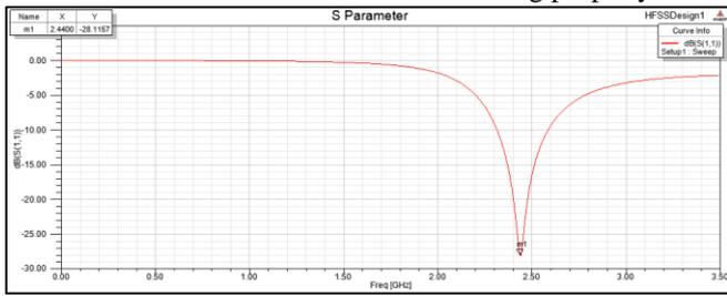
Fig. 5.3: Return Loss Vs Frequency
