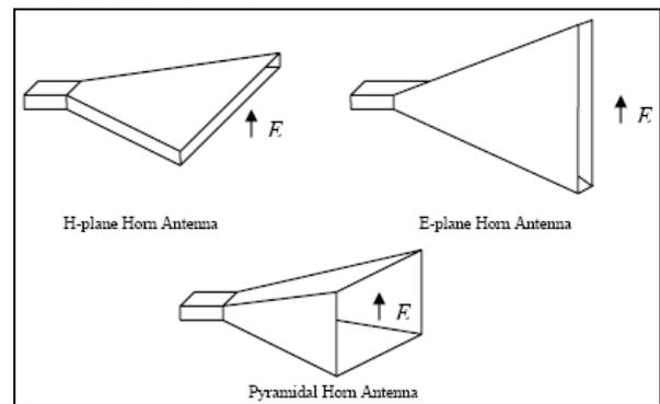
Fig. 2.5: Types of Horn Antenna
