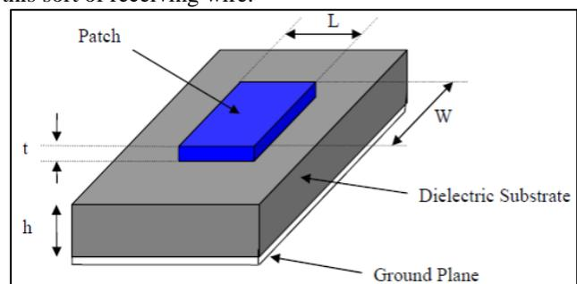
Fig. 2.6: Rectangular Microstrip Antenna
