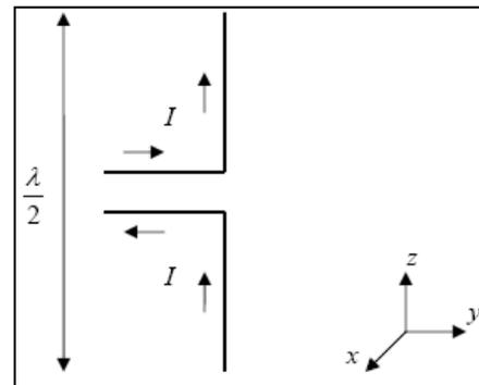
Fig. 2.1: Half-Wave Dipole
