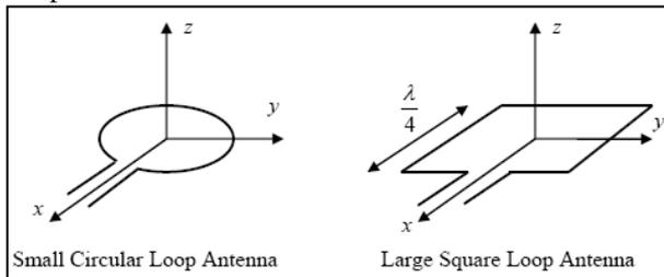
Fig. 2.3: Loop Antenna
