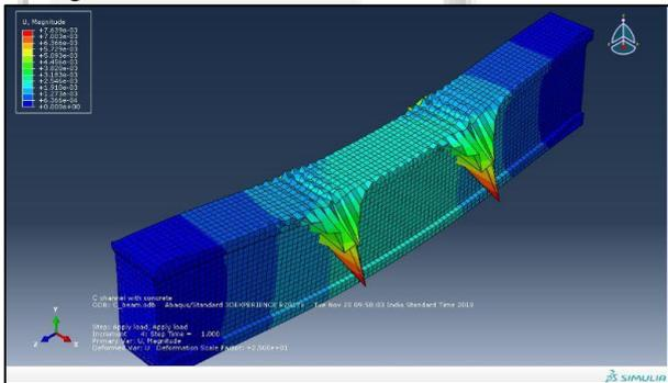
Fig. 5: Ultimate load failure in WOSC beam at 15kN
