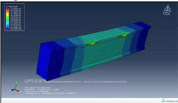
Fig. 6: Initial load failure in WSC beam at 10kN
