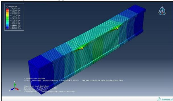
Fig. 4: Initial load failure in WOSC beam at 10kN
