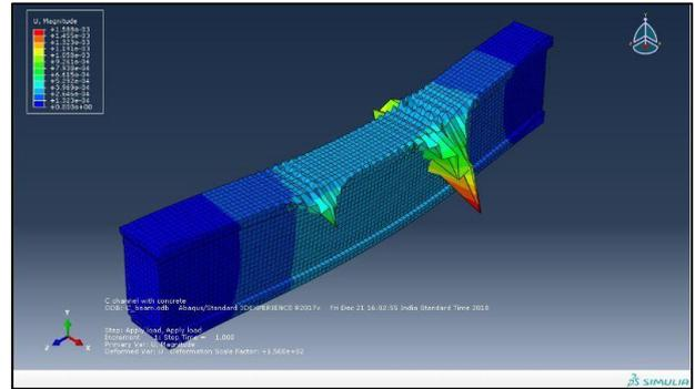
Fig. 7: Ultimate load failure in WSC beam at 26 kN
