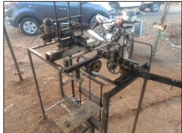
Fig. 1: Bar Cutting with Bending Machine
