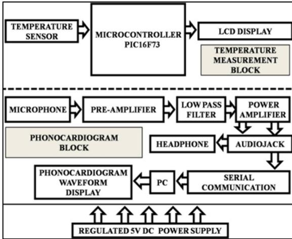
Fig. 1: Block Diagram representation of Phonocardiogram with Temperature Measurement
