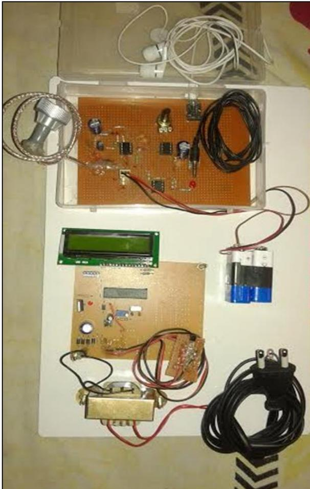
Fig. 4: Picture of the Phonocardiogram with Temperature Measurement
