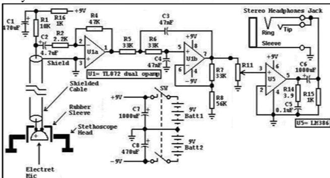
Fig. 2: Circuit Diagram of Phonocardiogram with Audio Output
