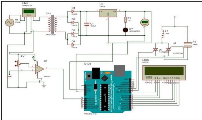
Fig. 2: Power quality improvement using by Static Var Compensator
