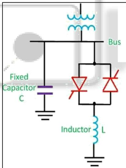
Fig. 3: Static Var Compensator
