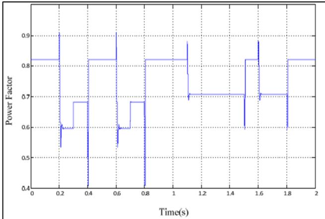
Fig 5. Power factor including fault load, no SVC
