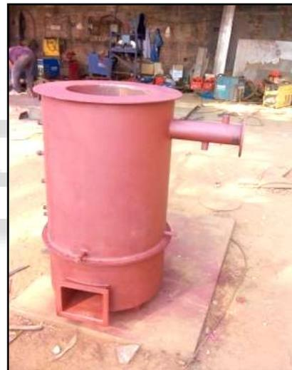
Fig. 7: Laboratory Scale Downdraft Biomass Gasifier
