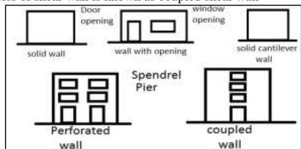
Fig. 2: Shear Walls- Solid, with Opening, Coupled
