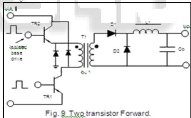
The two transistor version is popular for off-line applications. It provides higher output powers and faster switching frequencies. The disadvantages are again the extra cost of the higher component count, and the need for an isolated drive for the top transistor.
