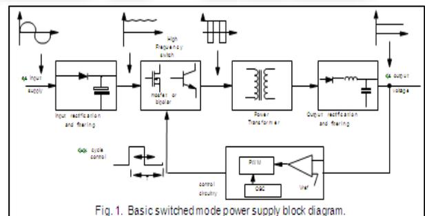
Fig.1. Basic switched mode power supply block diagram.
