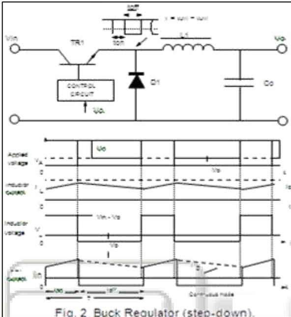
Fig. 2 Buck Regulator (step-down).
