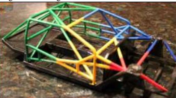
Fig. 1.6: ABS Rapid Prototype Roll Cage
