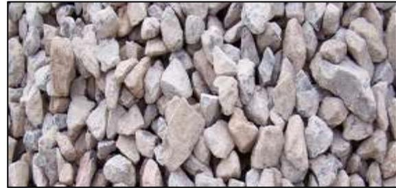
Fig. 1: Angular Aggregate
