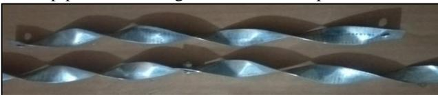
Fig. 3.2: Twisted Tapes ( $\gamma=5.0$ )
