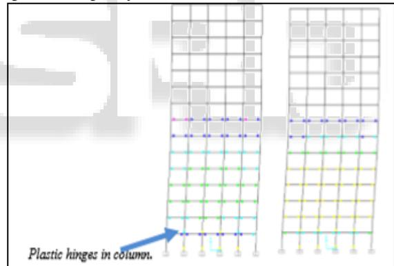
Fig. 6(a): Hinge formation By Elastic design approach
