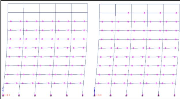
Fig. 4(b): Hinge formation in RCC
