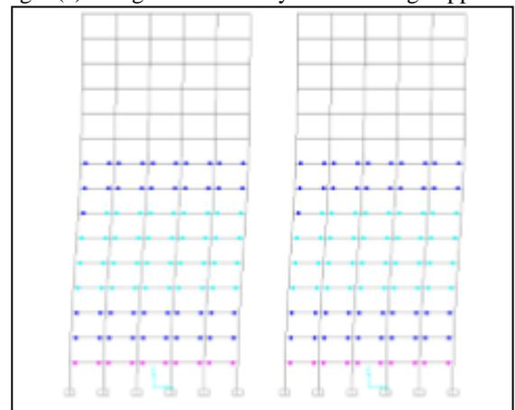
Fig. 6(b): Hinge formation by plastic design approach
