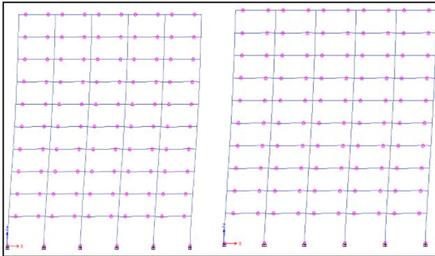
Fig. 4(a): Hinge formation in Composite
