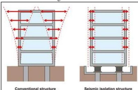
Fig. 1: Conventional & Seismic Isolation Structure
