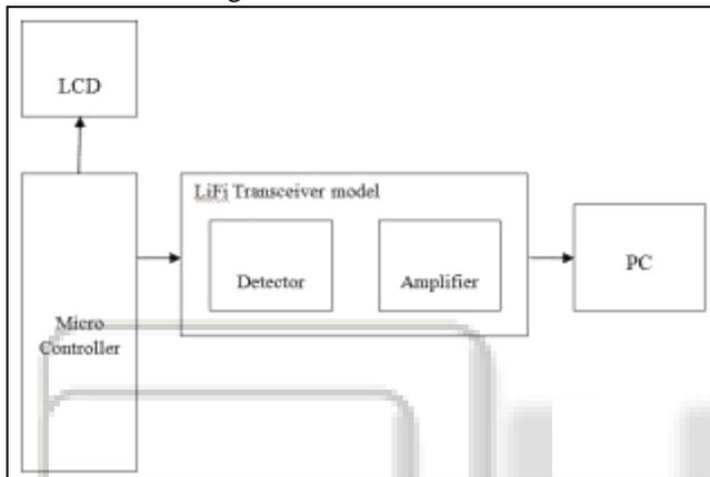
Fig. 2: Receiver section
