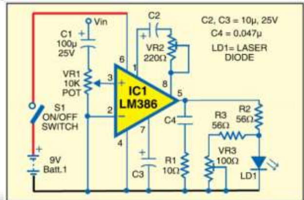
Fig. 3: Li-Fi Transmitter Circuit
