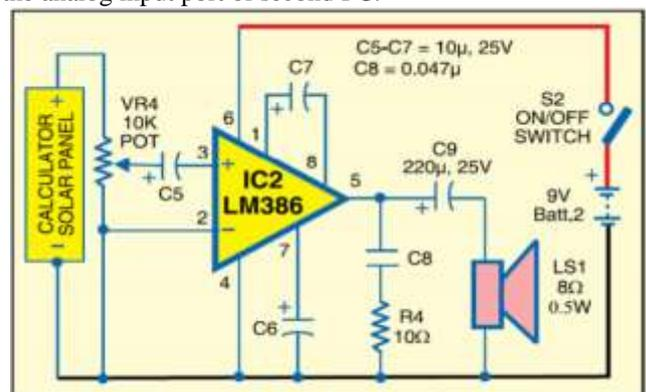
Fig. 4: Li-Fi Receiver Circuit
