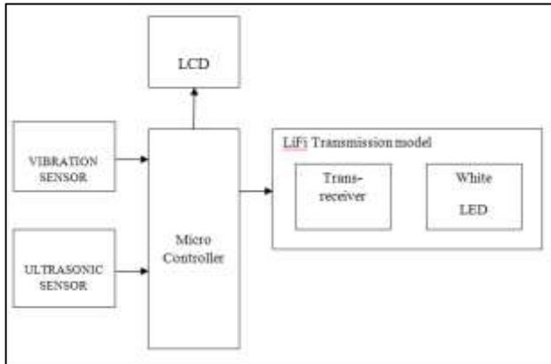
Fig. 1: Transmitter section
