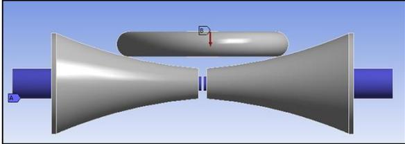
Fig. 5: Assembly of Toroidal CVT Model
