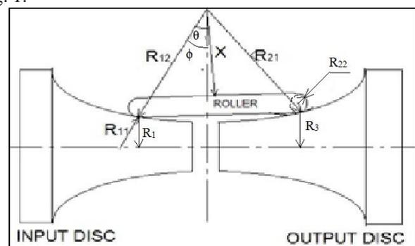
Fig. 1: Geometry of the Half Toroidal CVT
