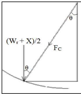
Fig. 2: Normal Force Acting On the Disc
