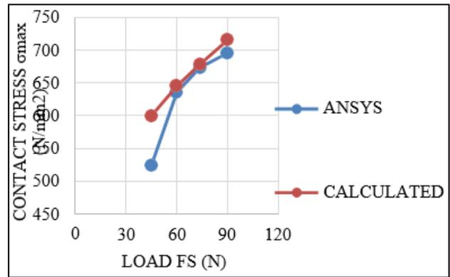
Fig. 6: (C) Comparison of Contact Stress Material 100Cr6/Si3Ni
