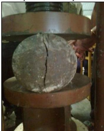
Figure: 4.3 Split Tensile Strength Test of Concrete
