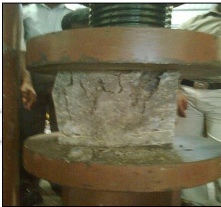
Fig. 4.1: Compressive Strength Test of Concrete
