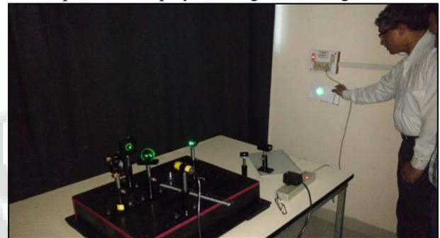
Fig.9 Hologram recording set-up
