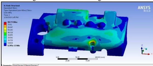
Fig. 7: Stress Results of Engine Cover
