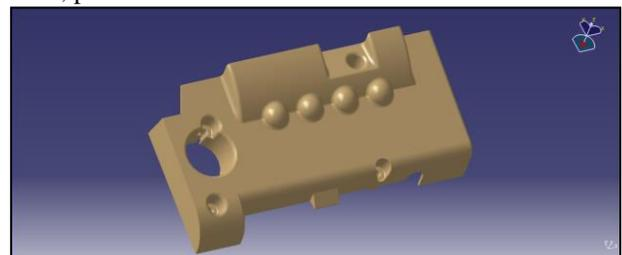
Fig. 1: 3D Modeling of Engine Cover
