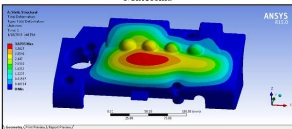
Fig. 6: Deformation of Engine Cover
