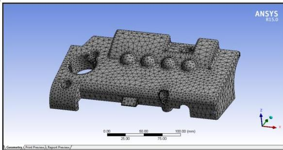
Fig. 2: Mesh Model of Engine Cover
