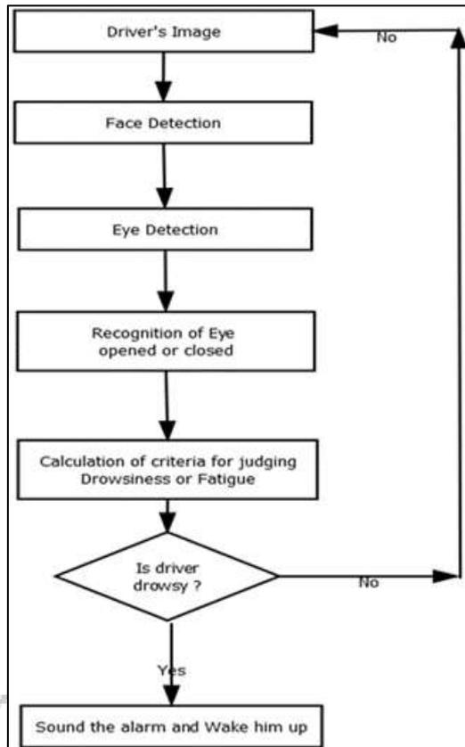
Fig. 1: Structure of Driver Fatigue Detection
