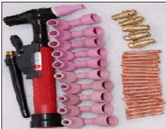
Fig. 1: Gas Nozzles
