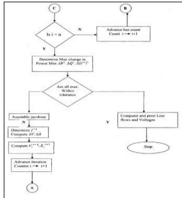
Fig. 2 Newton Raphson Load flow Analysis Flow chart
