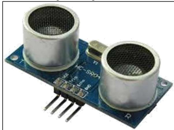
Fig. 3: Ultrasonic Sensor [13]
